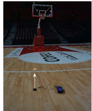
Horizontal illuminance (EH) measurement
