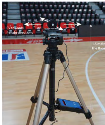
Vertical illuminance (EV) measurement
